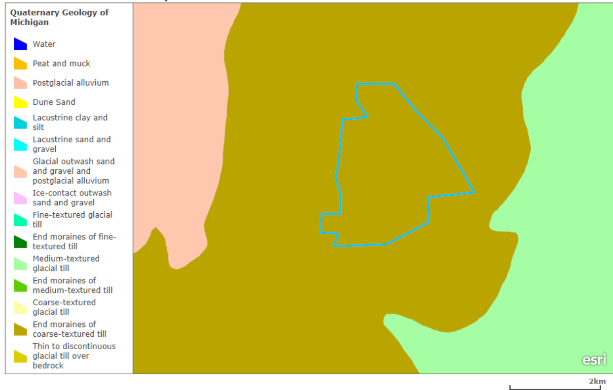
Figure 5. The overlay of feature layer "Quaternary Geology of Michigan" in ArcGIS confirms that the Bernard W. Baker Sanctuary is situated on an end moraine of coarse-textured till, with medium-textured glacial till to the east and glacial outwash deposits to the west and south.
